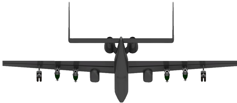
Figure 4.10: A-20 tail plane covering engine exhausts
