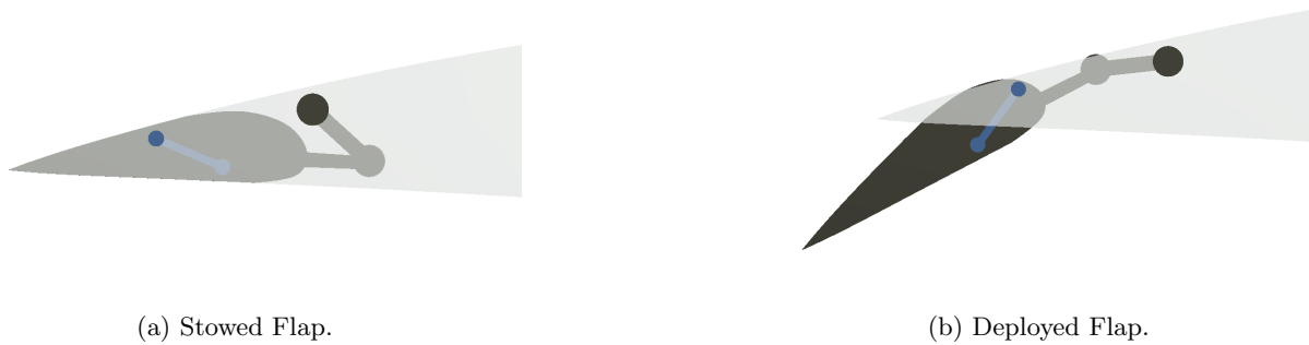
Figure 22: Example Flap Mechanism
