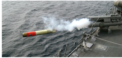
Figure 27: Compressed Gas Launch for a Torpedo [12]
