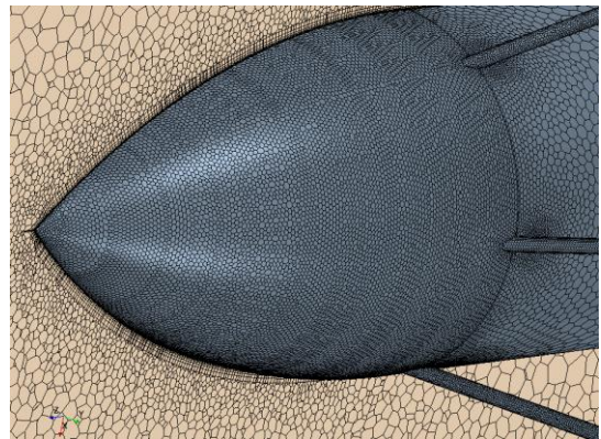
Figure 11.6: Surface Mesh and Prism Layers at Nosecone
