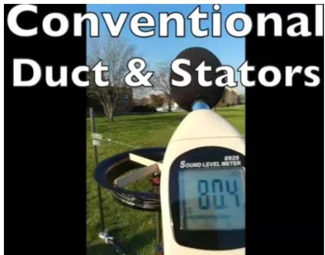
Figure 6.8: Conventional vs MicroStator Noise [43]
