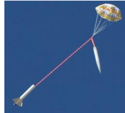
Figure 7.11: Emergency Parachute Deployment [47]
