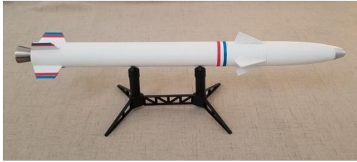
Figure 2.7: SAVAGE Kinetic Missile [11] 2.7 from a shoulder-launch platform (Figure 2.10). Electro-optical sensors guide the missile toward the target, which is then disabled upon impact. These re-usable rounds are effective against type 1, 2, and 3 UAVs up to a 5-kilometer range, but the ballistic nature of this system limits its availability and usefulness in populated areas.
