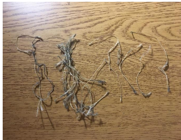
Figure 8.19 Burned and Frayed Kevlar Strands
