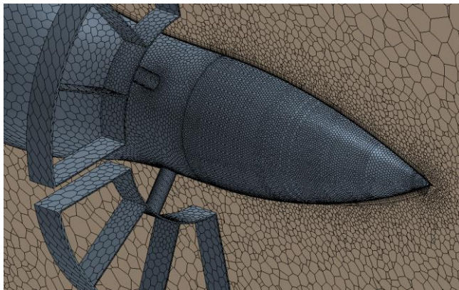
Figure 11.5: Surface Mesh and Prism Layers at Ballute and Grid Fins
