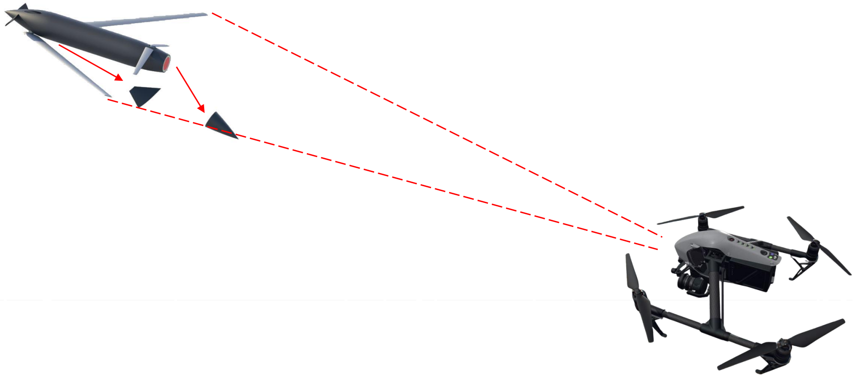
Figure 10.10: Valkyrie Discards Tail Cone and Cloth Wing
