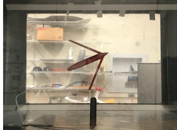
Figure 20.2.1: 100% Scale Wind Tunnel Model in KU 3 x 4' Tunnel
