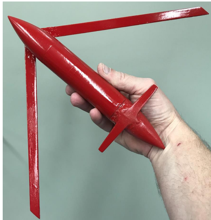
Figure 20.1.1: 100% Scale Wind Tunnel Model
