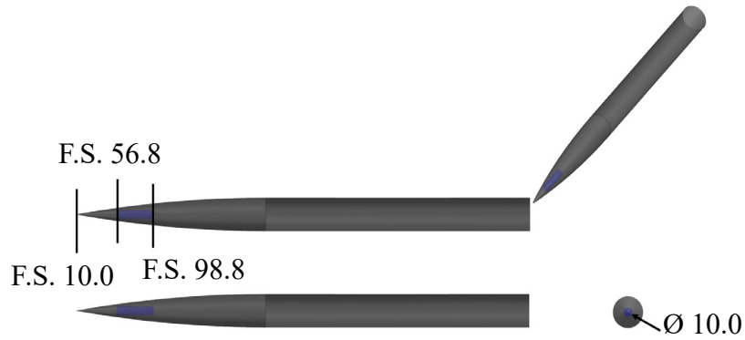
Figure 8.2: Payload Integration: 3-View and Isometric All Dimensions in Inches (Scale: 1:200)
