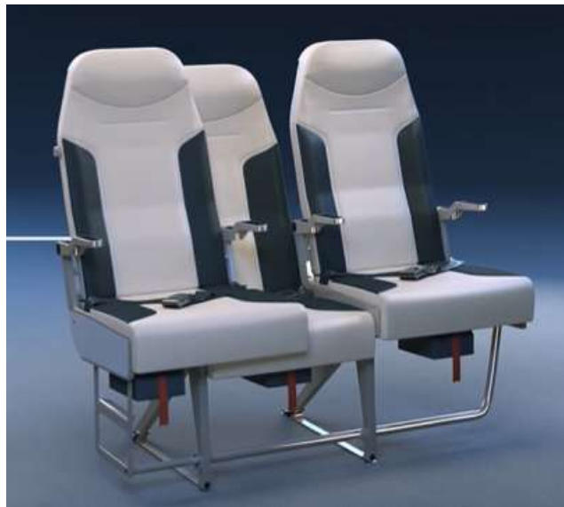
Figure 8 - Side Slip seating increases aisle width
