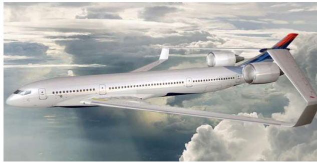
Figure 14 - Boxed Wing Design
