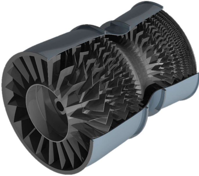
Figure 19: Compressor isometric view
