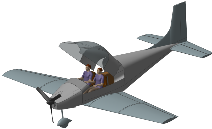
Figure 3.15: Access to the cabin
