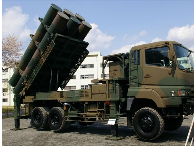
Figure 20.14: Active Hydraulics on Japanese Missile Launcher
