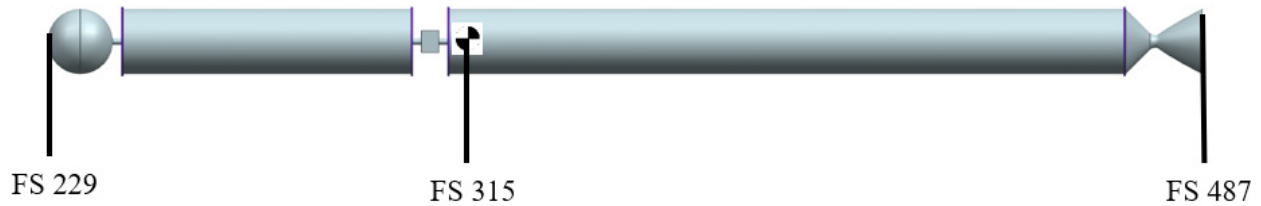
Figure 9.3: Hybrid Rocket CG Position Scale 1:40 (Units in Inches)
