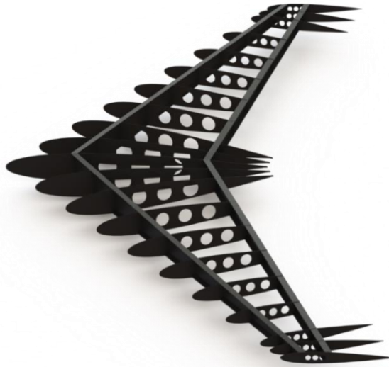
Figure 60. Condor X horizontal tail structure
