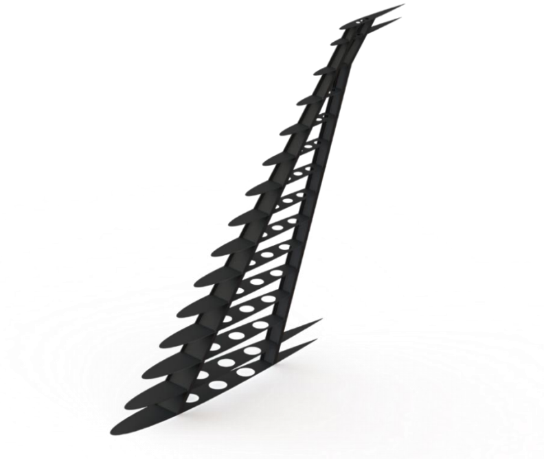
Figure 61. Condor X vertical tail structure
