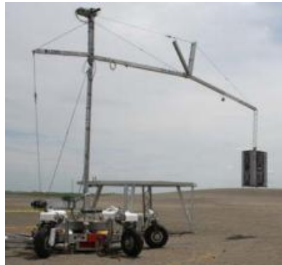
Figure 14. The LSMS and ATHLETE rover working together to perform offloading of simulated ISRU. This testing was done by NASA Langley at Moses Lake Washington [43].
