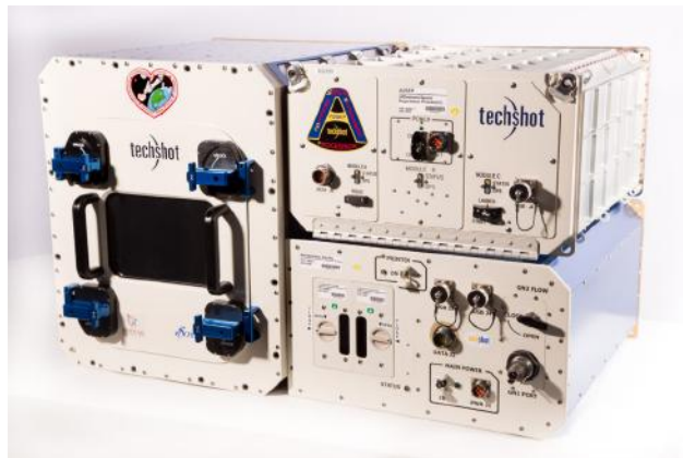
Figure 9. Biofabrication Facility onboard the ISS, a similar one will be used on at the lunar habitat to print tissue samples in various conditions.
