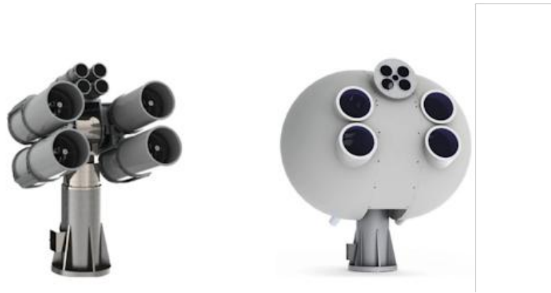
Figure 32. Diagram of the Lunar Laser Ground Terminal that shows all 8 telescopes, followed by an depiction of the telescopes encased in fiberglass layer.
