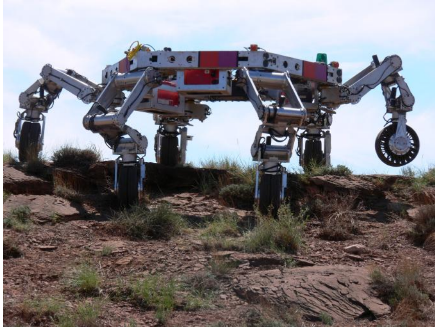
Figure 15. The ATHLETE rover is a six legged rover capable of stepping over rocks, which makes it very mobile and capable of climbing steep terrain [44].
