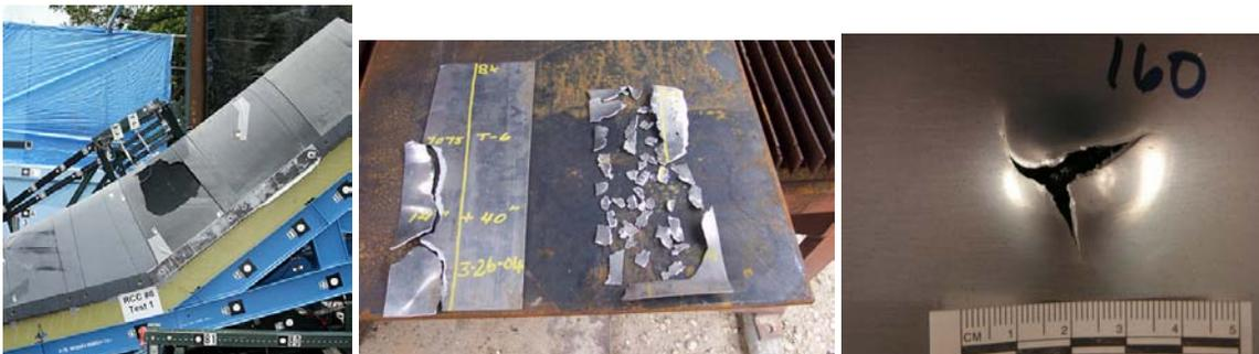
**Figure.** Impact tests on the space shuttle wing leading edge panels (left), components of the New Horizons third stage (center), and on an Altair pressure vessel wall (right).
