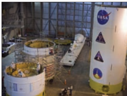
Ares I-X upper stage and launch abort system components are in place for stacking at Kennedy Space Center. Note the technicians working inside the 18-ft-wide upper stage section at left.
