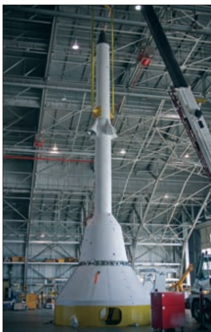
The "boilerplate" crew module and launch abort system for Ares I-X are stacked at Langley before transport to Kennedy.
