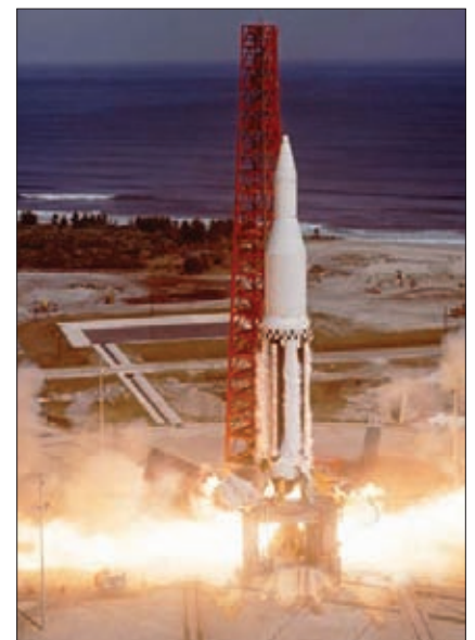
NASA tested the first three Saturn I boosters with live first and inert second stages. Here, the inaugural Saturn SA-1 lifts off from Pad 34 on Oct. 27, 1961. This first Saturn I was 162 ft high and weighed 460 tons at liftoff. Its eight H-1 engines generated 1.3 million lb of thrust. (NASA)
