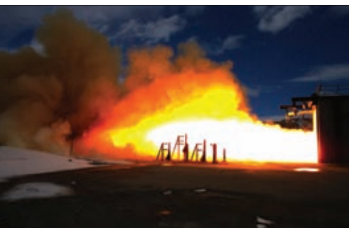
On March 10, 2009, ATK completed the successful test firing of the igniter that will be used to start Ares I's 5-segment, first-stage motor. The test, conducted at ATK facilities near Promontory, Utah, generated a flame almost 200 ft in length. ATK Launch Systems is the first stage prime contractor.
