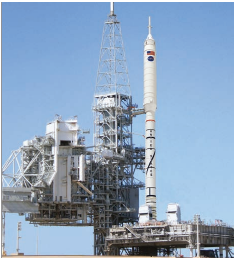
Ares I-X stands on Launch Pad 39B for a late summer 2009 launch. The test will use the existing shuttle service structure and mobile launch platform, as in this artist's depiction.
