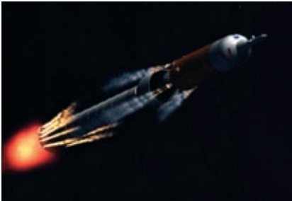
For Ares I upper stage separation, after RSRM thrust tail-off, a set of linear-shaped charges between the upper stage and first stage will fire, separating the metal between the first stage and the interstage. At the same time, 10 booster deceleration motors fire to pull the first stage directly backward, while eight ullage settling motors fire to push the upper stage forward. (NASA)
