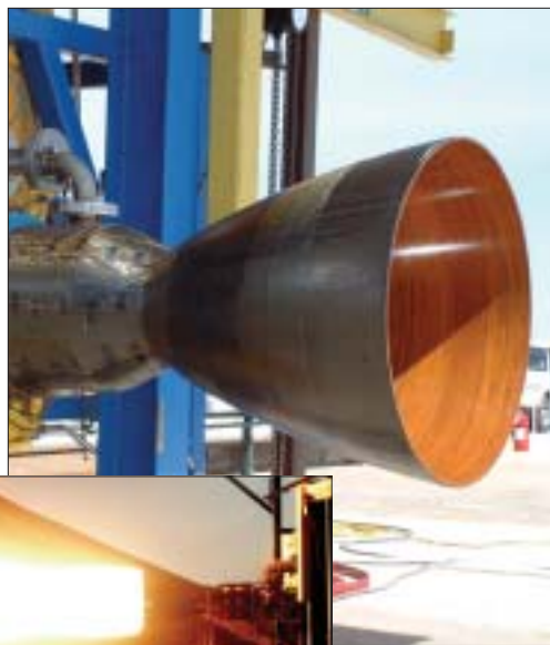
Kistler is planning to build two reusable engines by 2007, the Kestrel (below) and Merlin (right).
