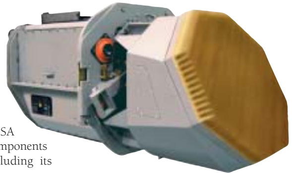
Raytheon's AN/APG-79 radar was developed for the Super Hornet, for new builds, and as a retrofit replacement for the mechanically scanned AN/APG-73.
