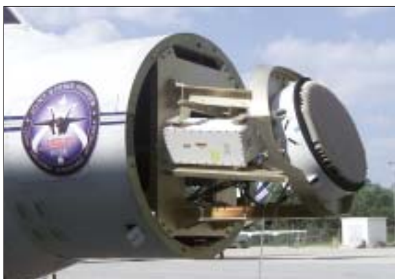
AN/APG-81 JSF radar was shown on Northrop Grumman’s BAC 1-11 test bed aircraft with its radome removed prior to its successful first flight test.
