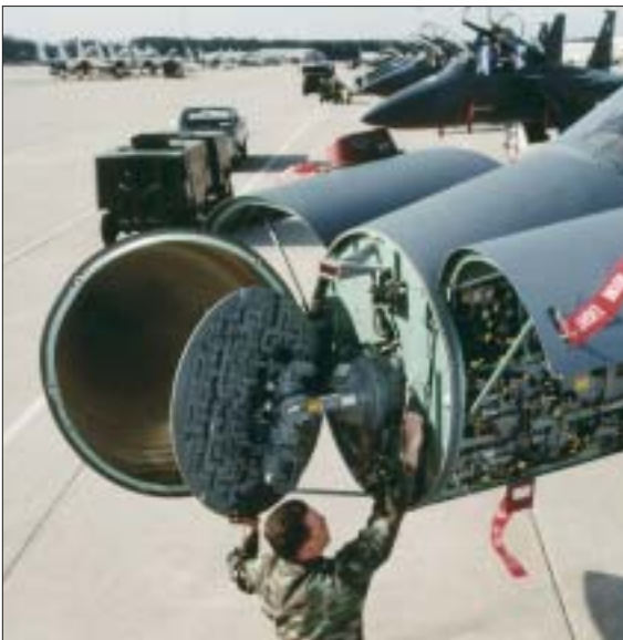
Raytheon's AN/APG-63(V) is the fire control radar for the F-15A/B/C/D.
