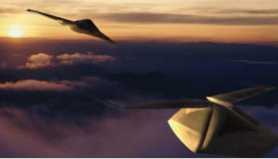
The Morphing UAV uses in-flight shape changing to provide different capabilities, as in the loiter and dash modes.
