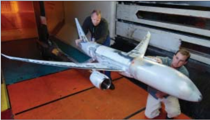
A 787 model is prepared for a series of tests at the Boeing transonic wind tunnel facility to help verify the performance of the airplane design during the highest speed portions of flight.
