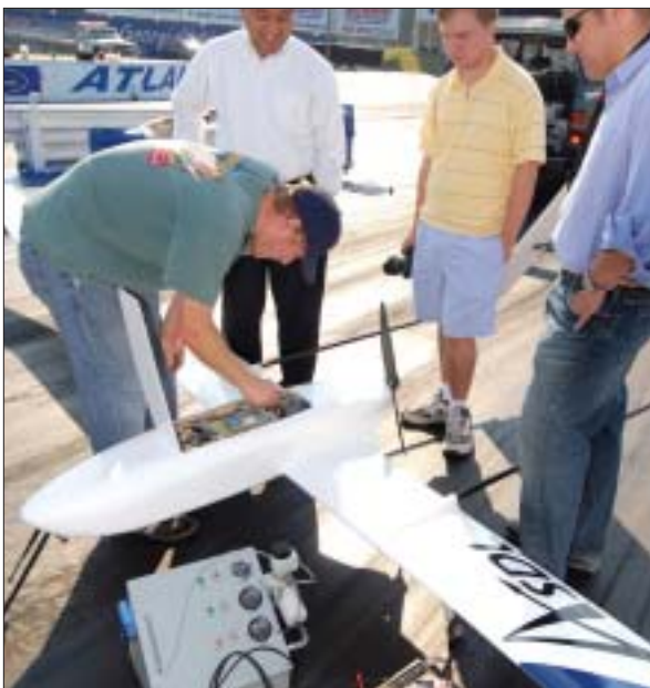
Thomas Bradley, David Parekh, Parker Parrish, and Adam Broughton remove the hydrogen tank from the fuel cell aircraft to refill it for flight.
