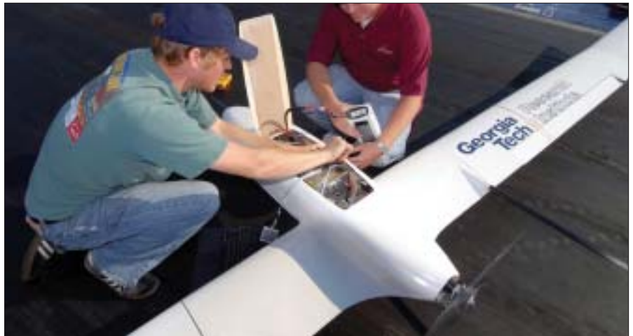
Thomas Bradley and Reid Thomas go through the procedure of starting up the Georgia Tech fuel cell aircraft during a test flight at the Atlanta Dragway. All photos by Gary Meek.
