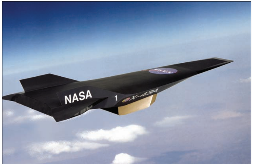
The air inlets on the X-43A—as well as the X-51A—feed air into rectangular combustors.
