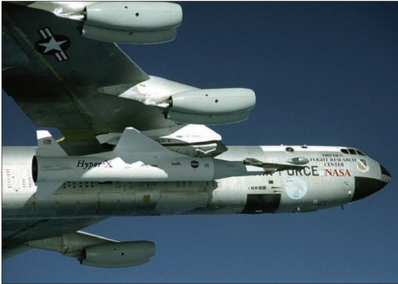
NASA's B-52B launch aircraft carried an X-43A hypersonic research aircraft attached to a Pegasus rocket to launch altitude. About an hour later the Pegasus booster was released from the B-52 to accelerate the X-43A to its intended speed of Mach 10. (Photo by Carla Thomas.)
