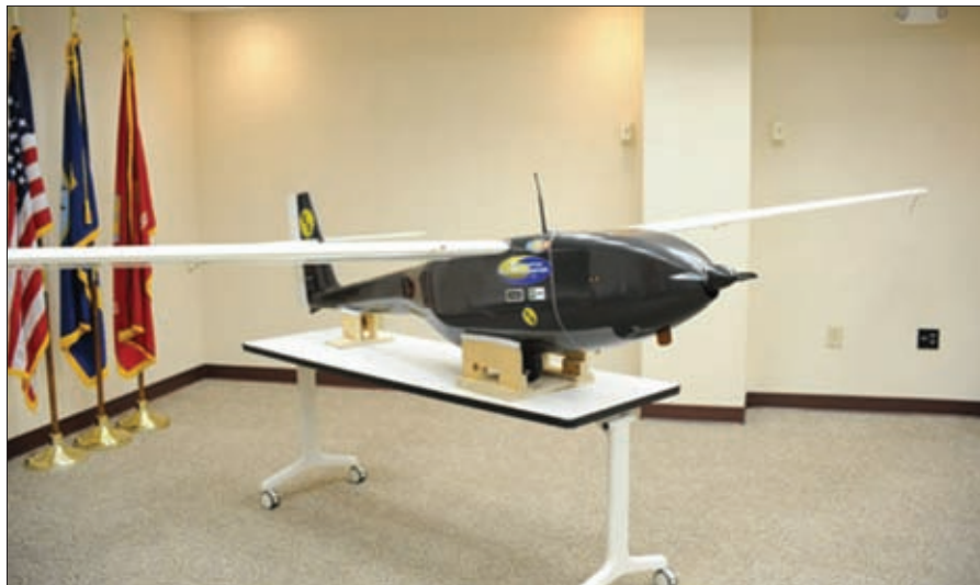
The Navy's Ion Tiger UAV operates with a high-powered fuel cell propulsion system. (Credit ONR)
