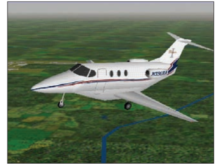
The Premier I features a composite airframe.
