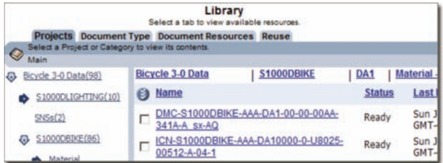
A basic library screen indicates the status of the data modules or documents that have been entered in the system.
