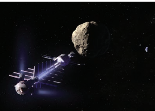
Astronauts Ed Lu and Stan Love at JSC devised the gravity tractor concept, a 20-ton nuclear-electric spacecraft that can tow a NEO by simply hovering near the asteroid. The steady thrust would gradually and predictably alter the course of the tug and asteroid, coupled by their mutual gravitational attraction. Credit: Dan Durda.
