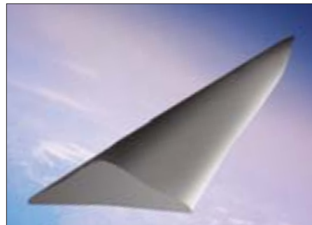
An enhanced CAV is meant to glide for 9,000 mi. along-track and 3,000 mi. across-track over 3,000 sec.
