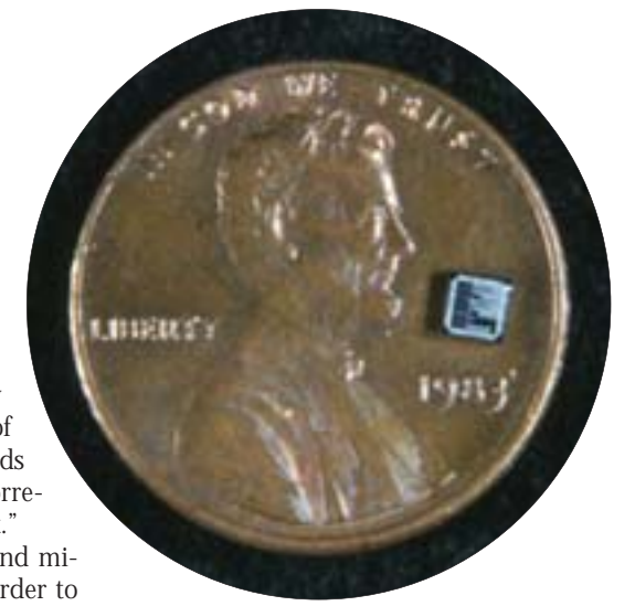
Integrated circuit microluminometer measures only 2×2 mm.
