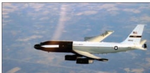
Big Crow No. 38050 is one of two identically named NC-135Es, based at Kirtland AFB, that served as a surrogate target for the ABL’s two illuminator lasers.
