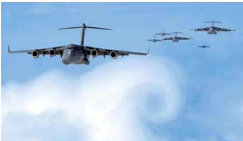
Using twisterons on transport aircraft could result in significant fuel savings. Here the right-hand wingtip vortex is outlined in the cloud below and aft of the lead aircraft.
