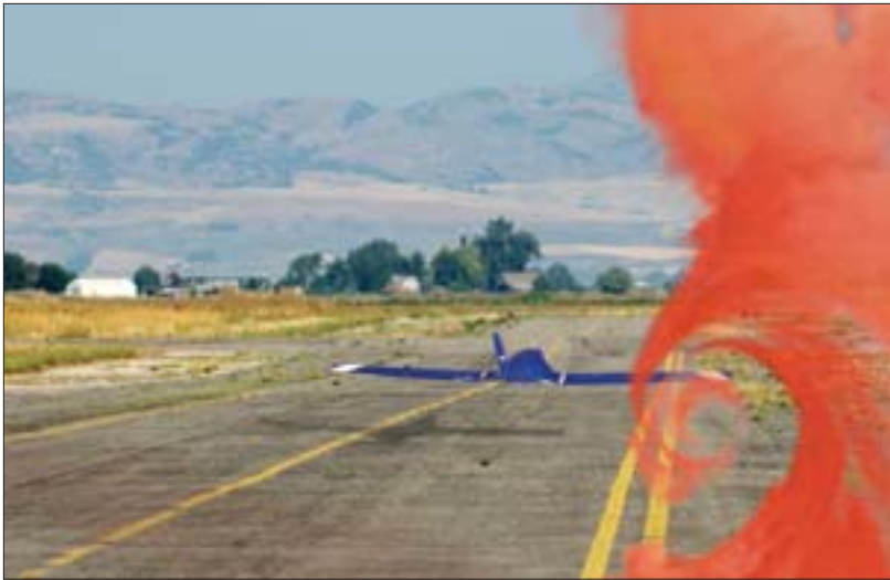
This prototype aircraft has operational twisterons; the wingtip vortex responsible for induced drag is shown in red.
