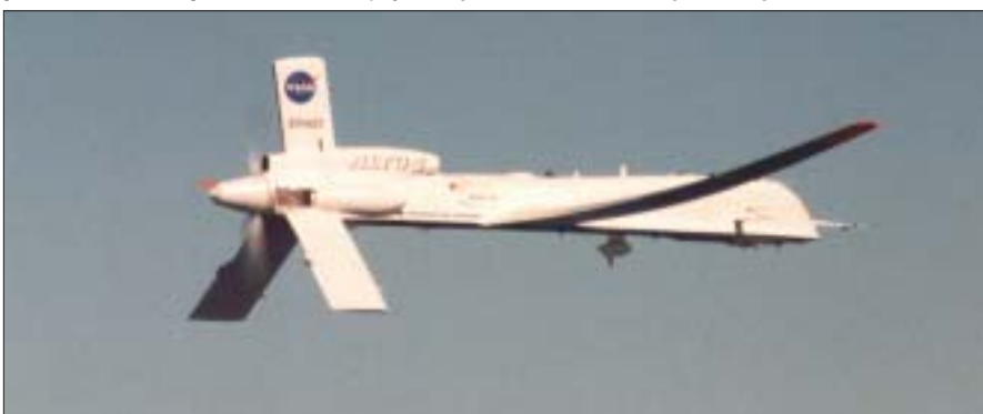
The ARM-UAV program used the Altus UAV for nine science flights that studied the role of clouds in global climate change. Altus carried a payload of 390 lb to altitudes of 50,000 ft or more.
