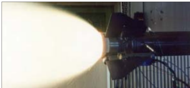
Bayern-Chemie/Protac's rocket-ramjet propulsion system for Meteor is powered to transition velocity by an integrated nozzleless booster motor.
