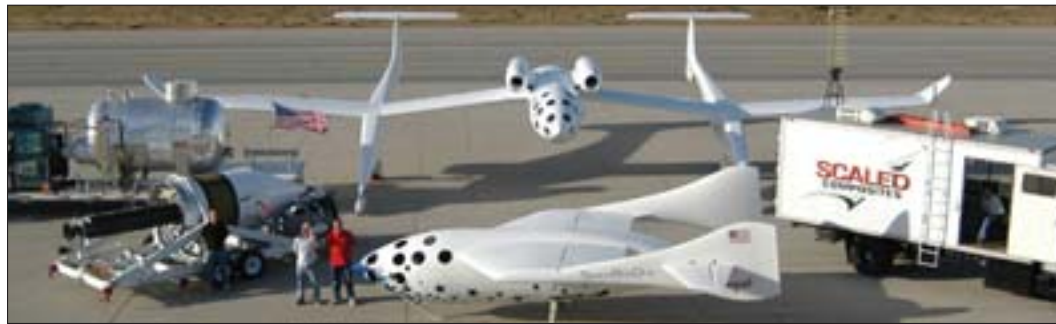
The elements of SpaceShipOne include the subsonic mother-ship, called White Knight (top) and the rocket-powered upper stage, dubbed Tier One.
