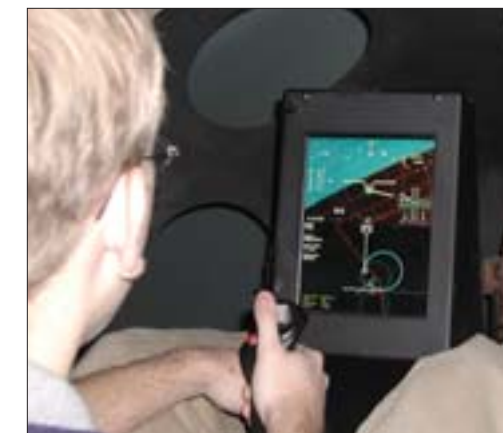
The innovative navigation and display system comprises a GPS/inertial navigation and attitude reference unit and a pilot's display with a single large LCD screen.
