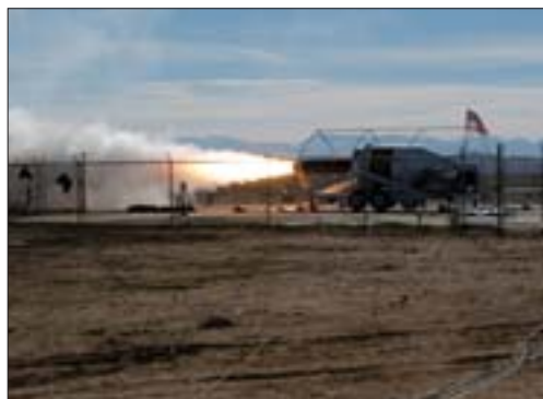
A hybrid rocket was chosen for the spacecraft, and it has undergone broad test firing.
