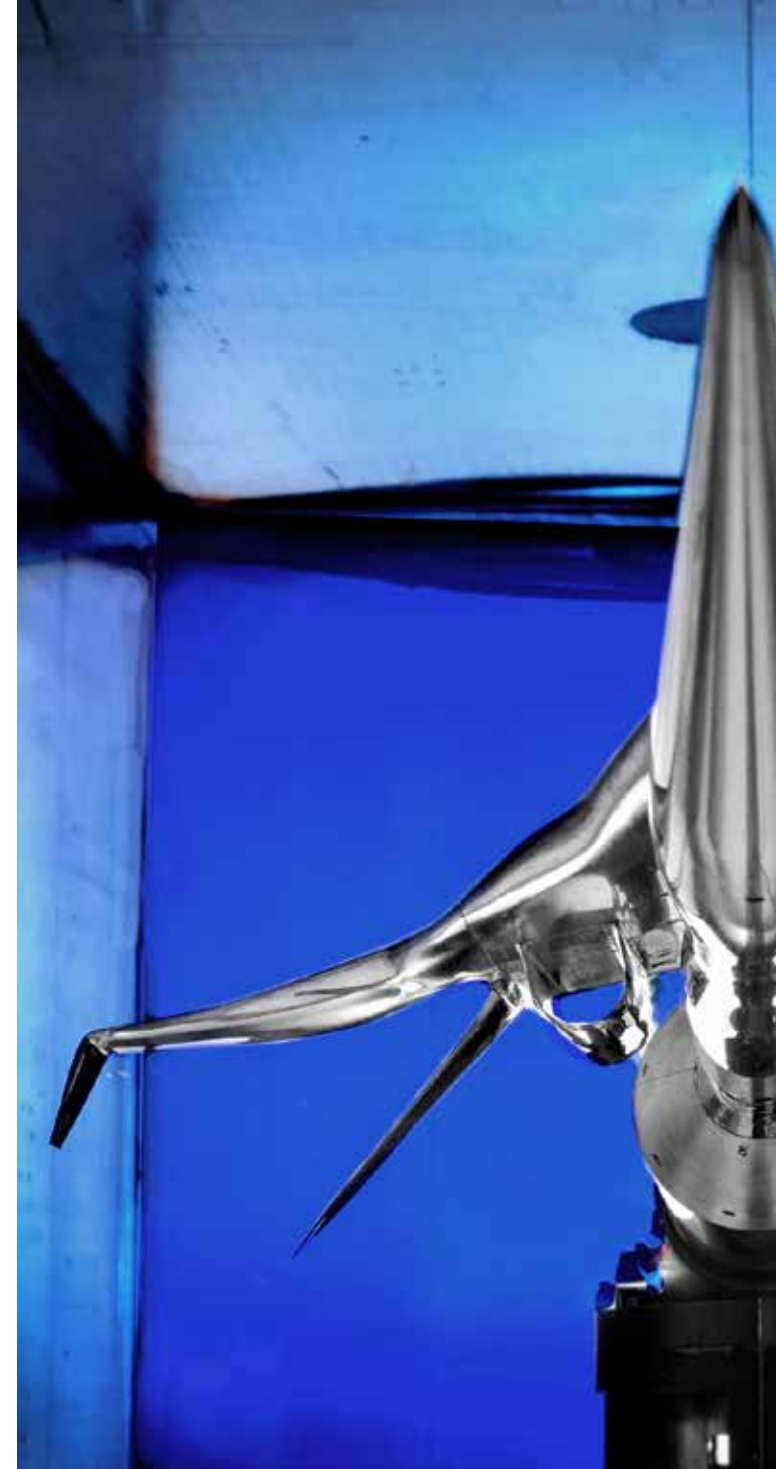
A wind tunnel test model for a Boeing supersonic aircraft Credit: NASA/Boeing
