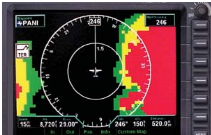
The FAA's Capstone program, which features a multifunction display, realized some safety benefits this year.
