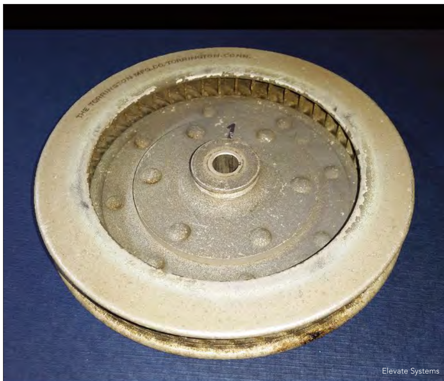
The 1950s-era impellers for B-52s were made of thin sheet metal folded like origami.
