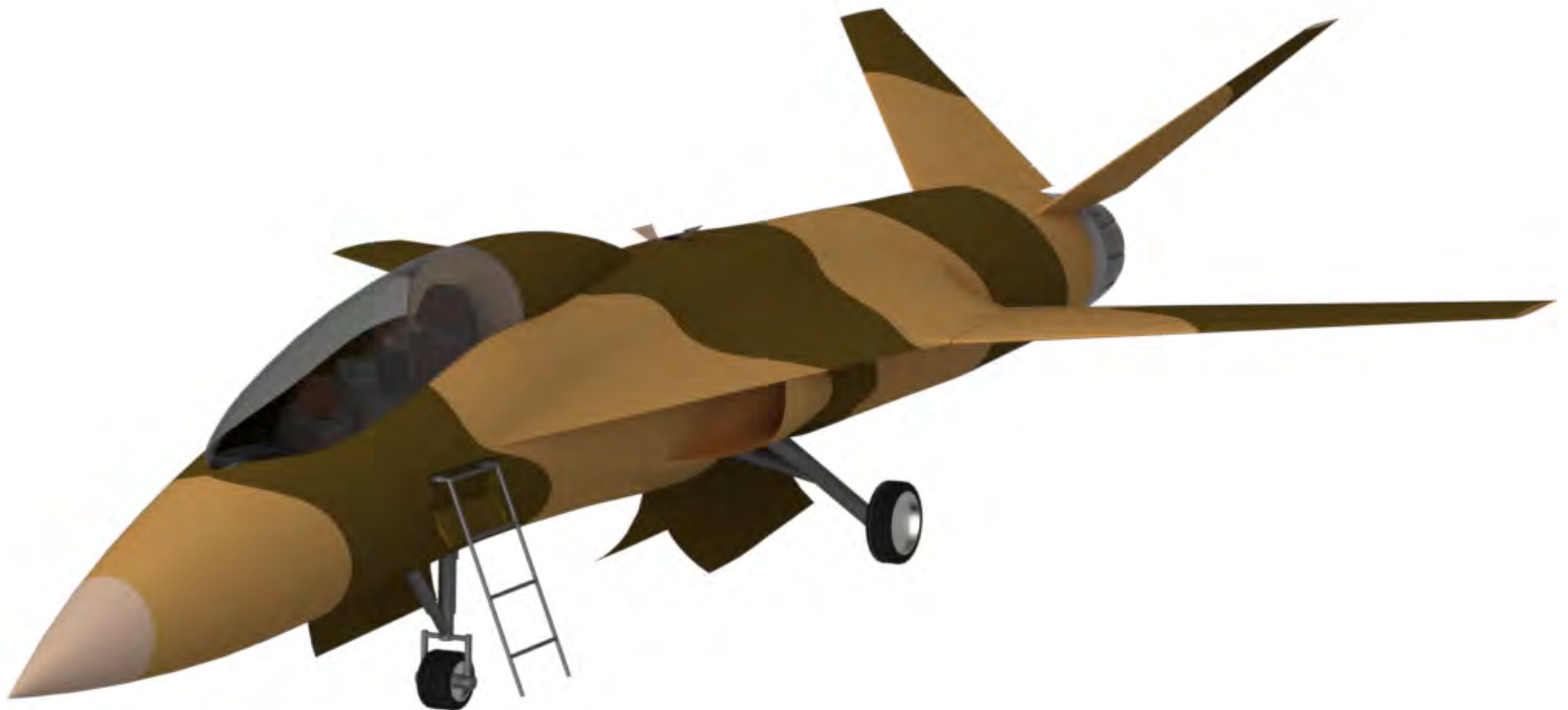
Figure A.4: Global view of the Coyote with the refuel hookup and the cockpit access ladder.
