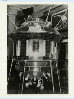
spacecraft of just less than a quarter of sea-level atmospheric pressure as a compromise between the needed structural strength and the issues caused by the behavior of materials in a vacuum. The shape of the spacecraft (seen on the right) reflects its pressurization.
