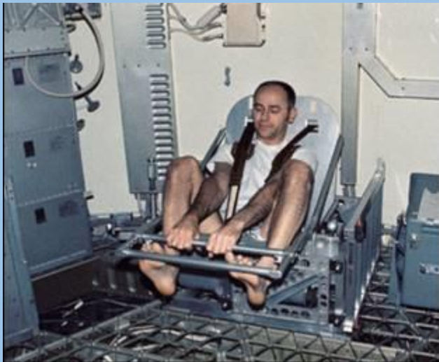
Bean using the BMMD to measure his body weight
