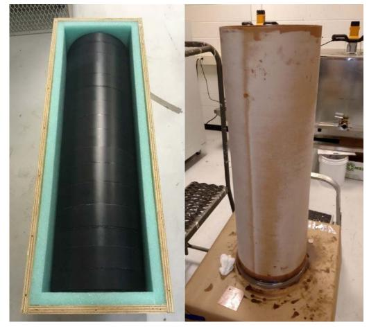
Figure 8 Multi-segment fuel grain (left) and multi-segmented fuel grain in a phenolic tube (right). [19]
