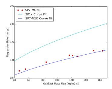
Figure 2 Comparison of Regression Rate Data for SP7/MON-3 With the Curve Fits for SP7/N<sub>2</sub>O and SP1x/N<sub>2</sub>O [10]
