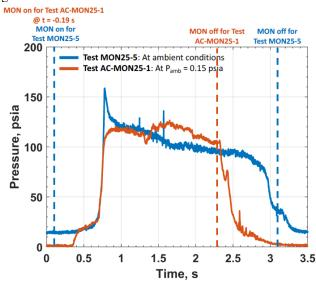
Figure 23 Purdue University Ground and Altitude Chamber (AC) Start Hypergolic Ignition Tests.
