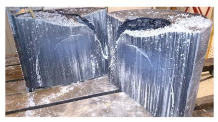
Figure 7 End Cooler technique fuel grain cut in half
