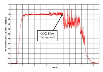
Figure 4 Non-Dimensional Chamber Pressure for Test MAV\_11\_19[12]
