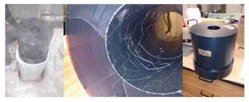
Figure 9 Processing in the -40C Freezer(left), cracks from warm insulator assembly(middle) and replacement segment (right) for Whittinghill Motor B (FT04)
