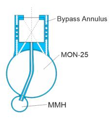
Figure 15 Cross section view of a hypergolic MON-25/MMH igniter concept.[21]
