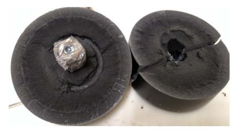
Figure 6 Early grain casting showing a mandrel design and grain cracking and voids
