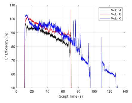
Figure 19 Whittinghill Aerospace C\* Efficiency for Motors A, B and C.[22]
