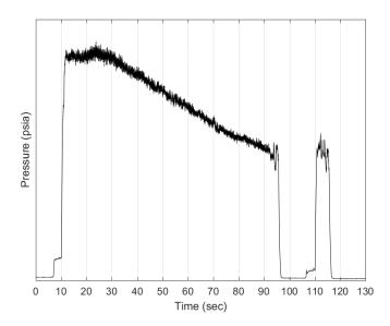
Figure 12 Whittinghill Aerospace FT01 Chamber Pressure [20]
