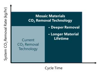
ultra-high capacity under dilute (<1%) CO<sub>2</sub> concentrations – up to three times the CO<sub>2</sub> capacity of existing materials. The combination of ultra-high capacity and rapid adsorption means a reduction in both capital and operating expenses for life support and other dilute CO<sub>2</sub> removal systems.
