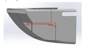
If the problem lies in complex geometry, can we provide a tool that would help the tech inspection to verify the maximum longitudinal direction of the hatch? For example a »positive« volume that takes up the space of the hatch opening, or something similar– the volume could be easily laid on one side and measured.
