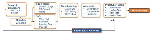
Figure 4.1 – Manufacturing Plan
