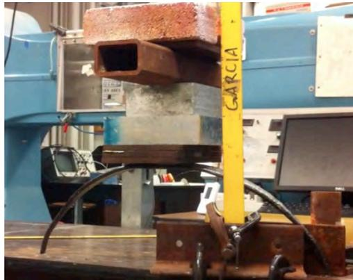
**Figure 8.2: Main gear static load test**
