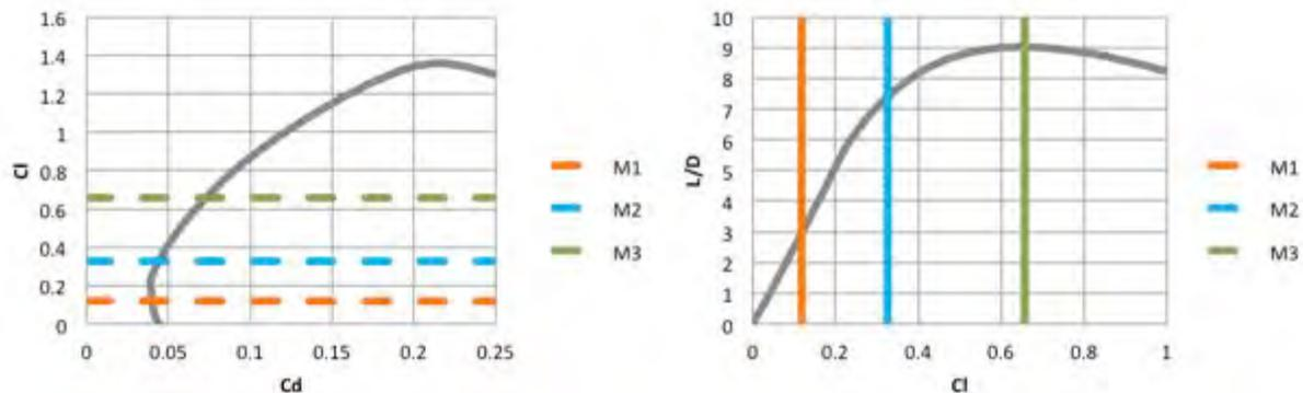
Figure 4.8: Left: Drag polar of the entire plane. Right: Lift to drag ratio of the entire plane
