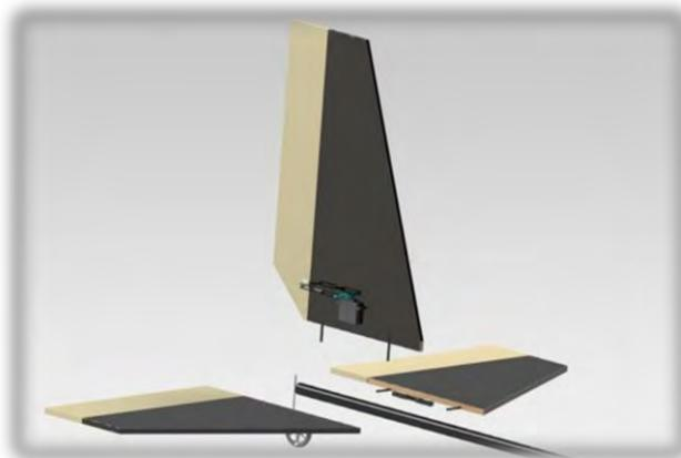
**Figure 26: Empennage Attachment**
