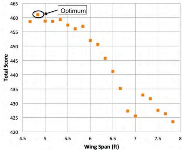
Figure 4.7: Effects of span on total score for final plane design
