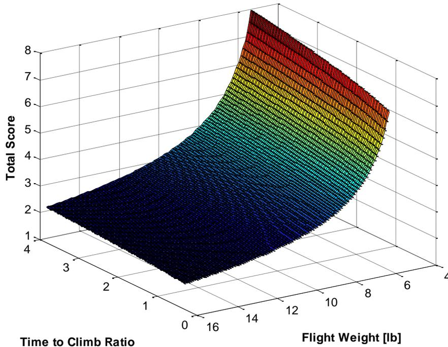
**Figure 4: Effect of Time to Climb Ratio and Flight Weight on Total Score**
