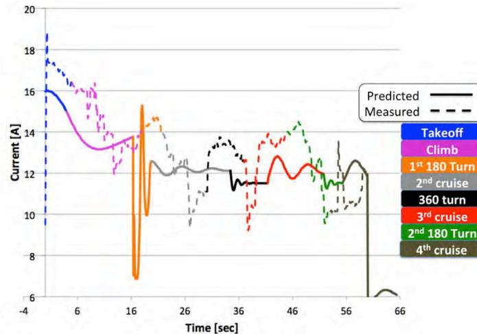
**Figure 8.4: Predicted and measured current for mission 2 lap 1**
