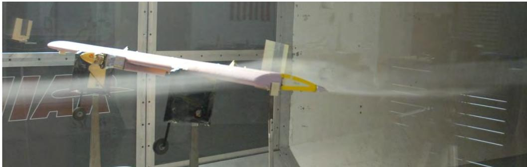
**Figure 51: Smoke Visualization in the 7x10ft Walter H. Beech Wind Tunnel Test**
