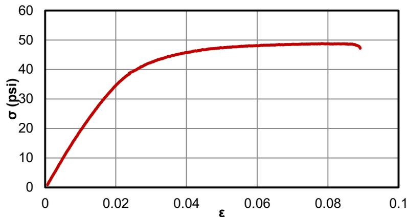
**Figure 55: XPS Foam Stress and Strain Plot**
