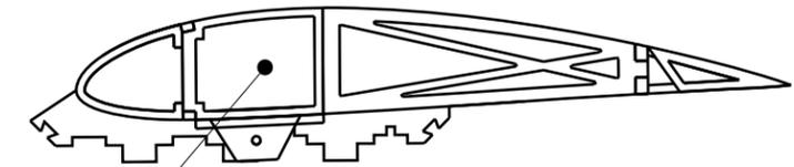
2L WATER PAYLOAD IN HOLLOW BOX SPAR WING SIDE VIEW
