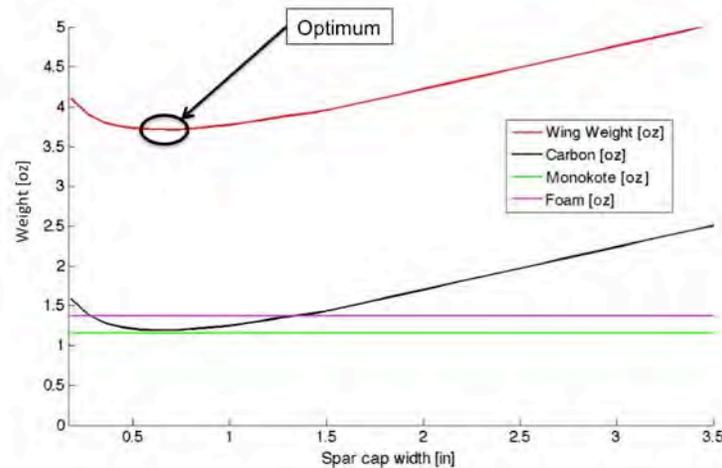
**Figure 5.7: Effect of spar cap width on the total wing weight**
