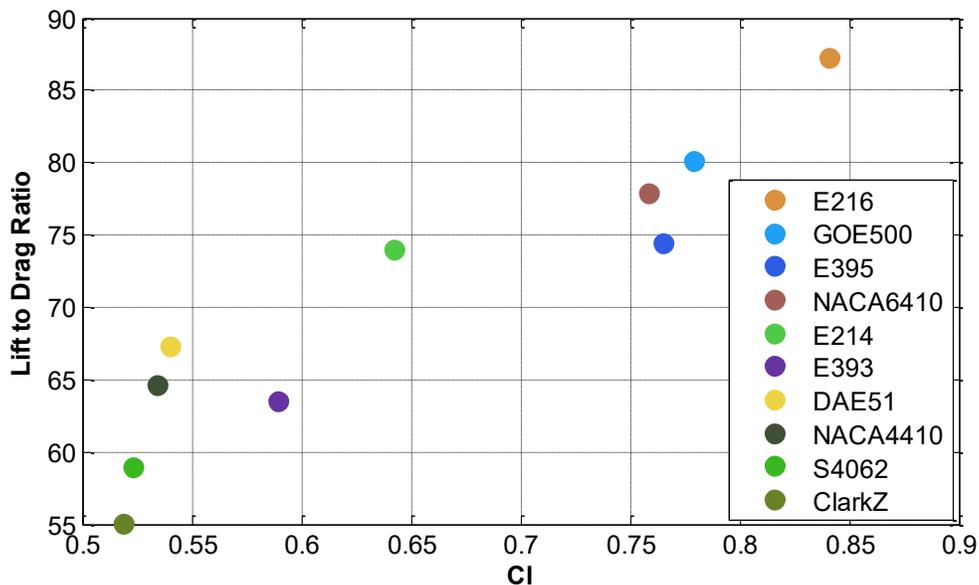
**Figure 6: Lift-to-Drag Ratio versus Coefficient of Lift for Various Airfoils**
