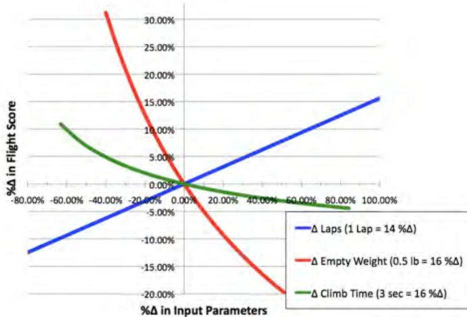
**Figure 3.3: Impact of change in parameters on the total score**
