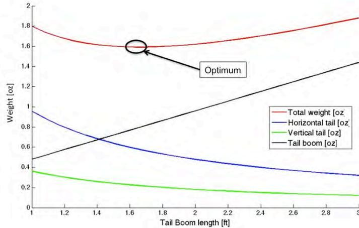
**Figure 5.10: Effects of tail boom length on the total weight of tails and tail boom**
