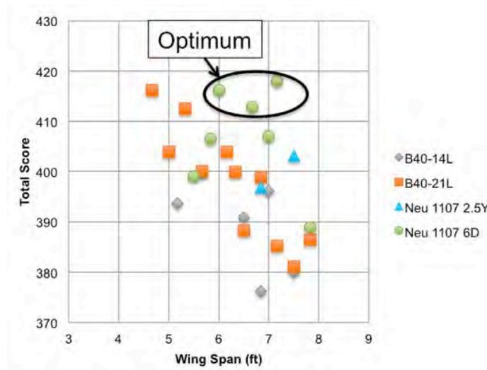
Figure 4.5: Effects of motor selection and span on total score
