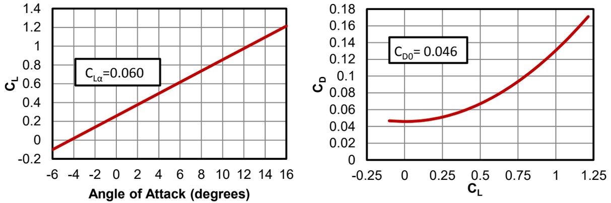
Figure 16: Predicted Lift Curve Slope and Drag Polar
