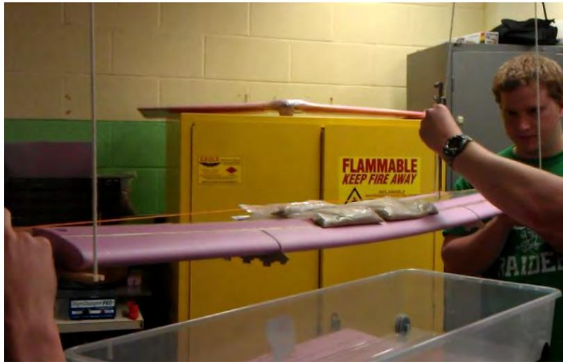
**Figure 56: Structural Deflection Test**
