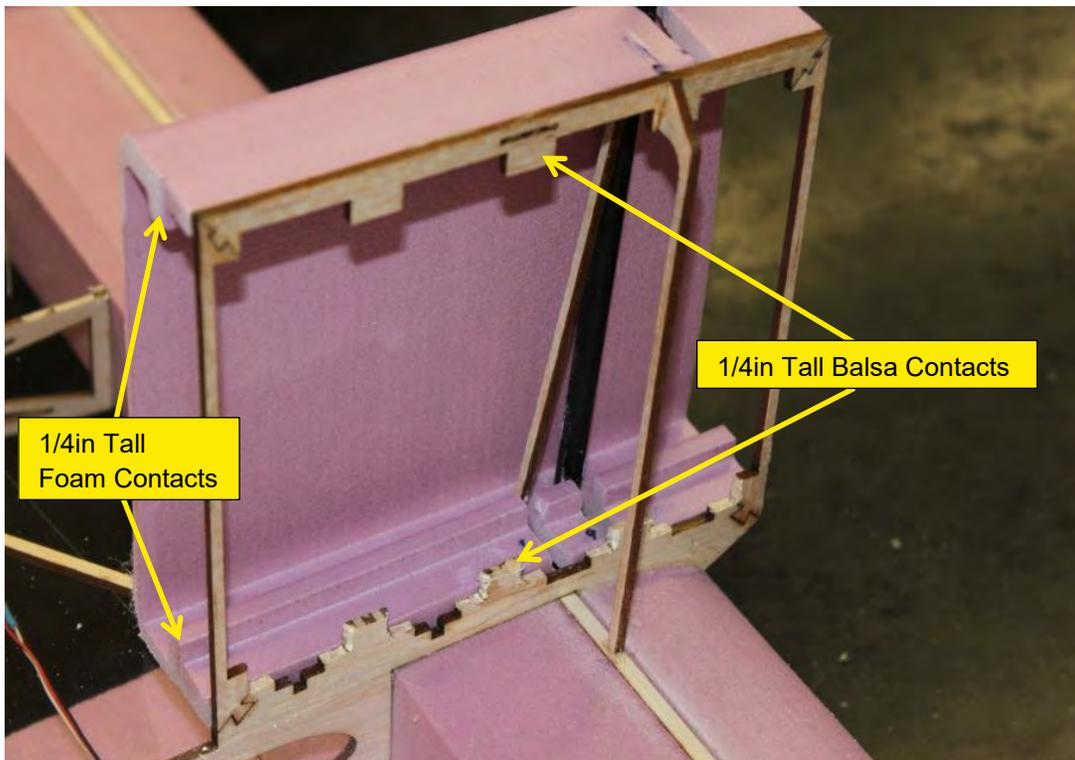
**Figure 37: Pod Shown Inverted and Without Fairings**
