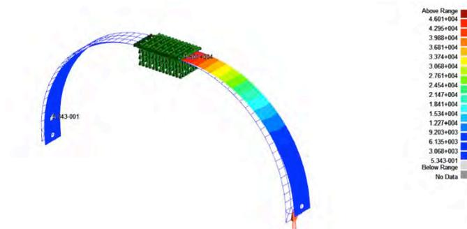
**Figure 5.12: Compressive stress (psi) for one wheel landing**
