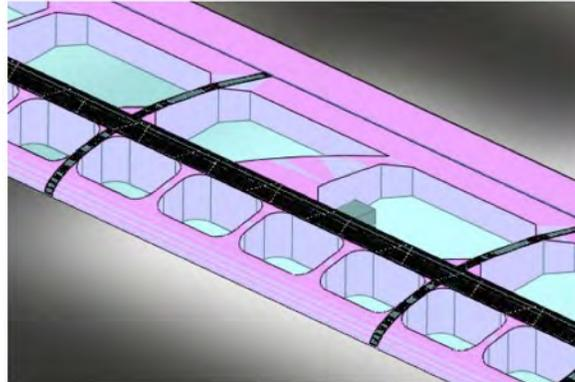
**Figure 5.6: Hollow foam and carbon fiber wing**
