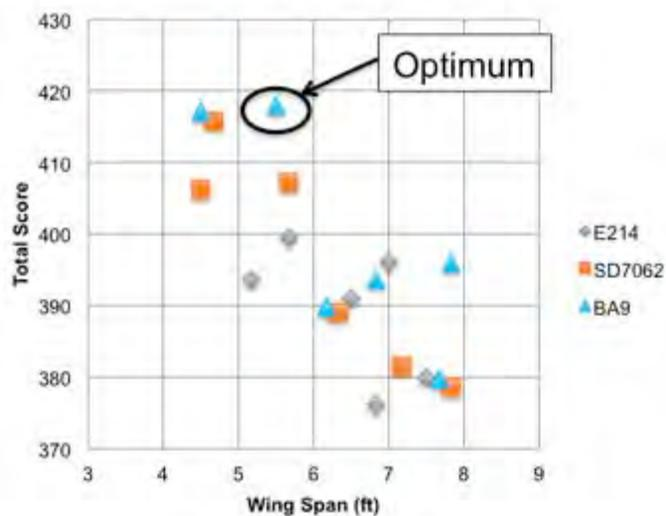
Figure 4.4: Effect of airfoil selection and span on total score
