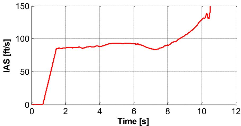
**Figure 36: Calibration Data for Pitot Probe**
