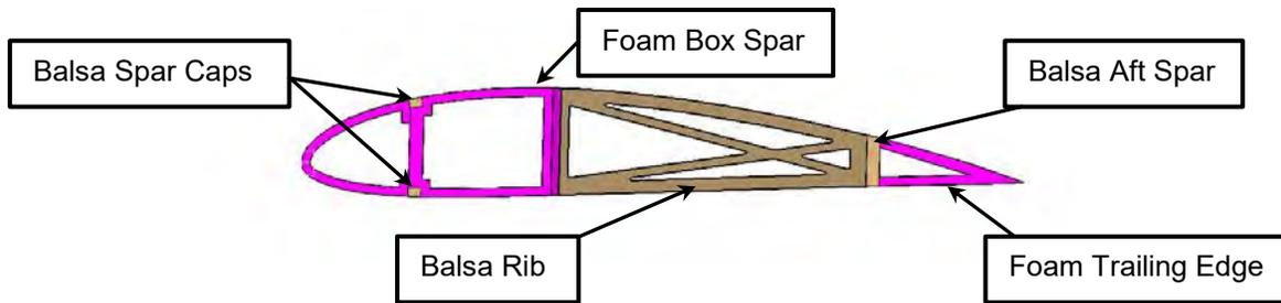
**Figure 28: Wing Structural Cross Section**
