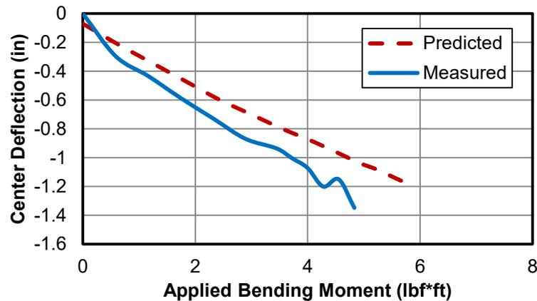
**Figure 64: Structural Deflection Comparison**
