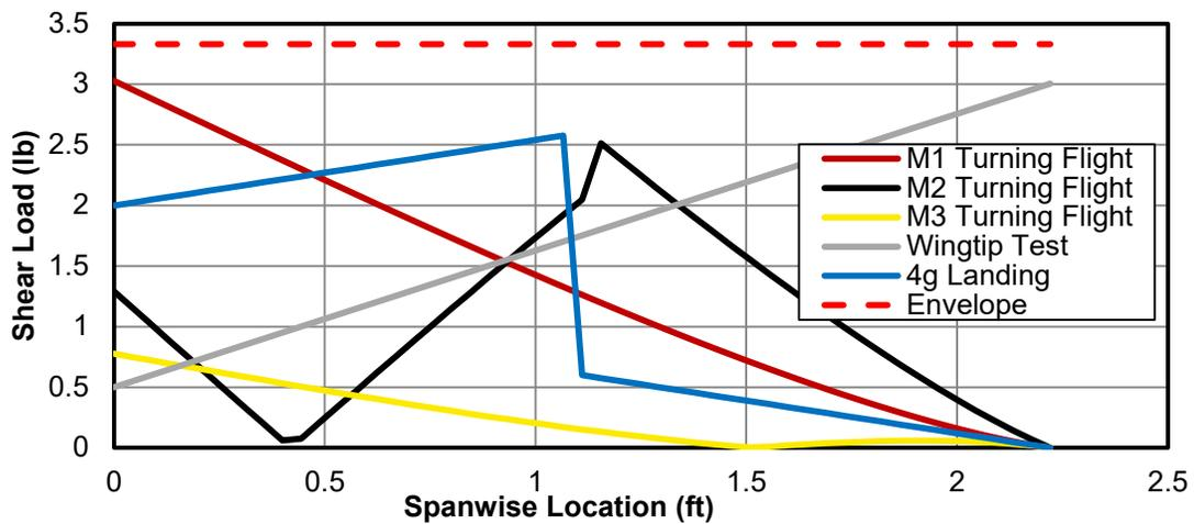
**Figure 29: Shear Load Envelope**
