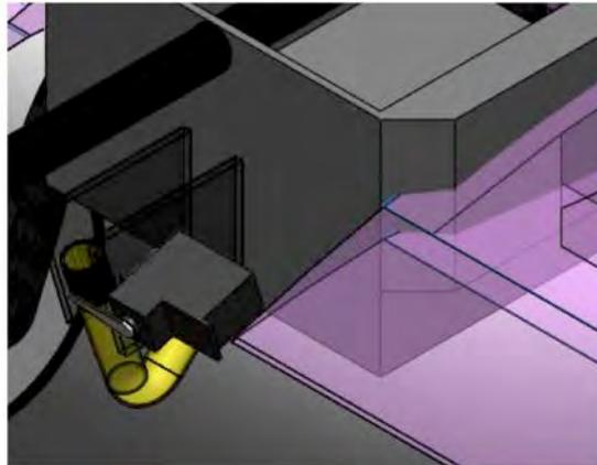
**Figure 5.4: Water tank release system**
