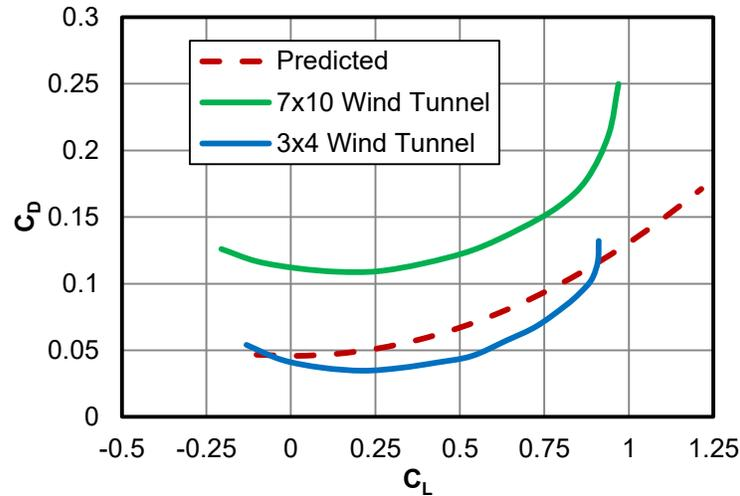
**Figure 62: Drag Polar Comparison**
