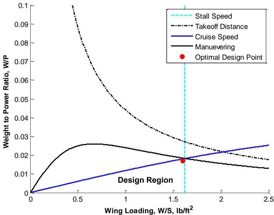
Figure 5: Performance Constraint Plot
