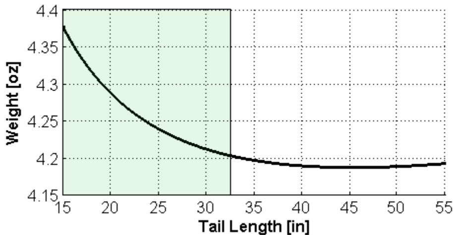
Figure 8: Tail Mass as a Function of Tail Length for a Constant Tail Volume
