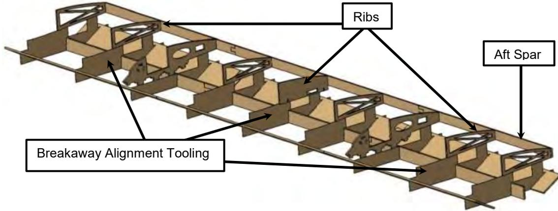
**Figure 47: Breakaway Rib Jig**
