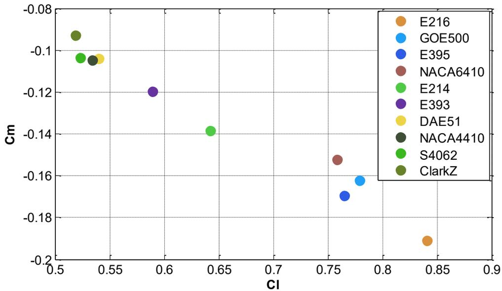
**Figure 7: Coefficient of Moment versus Coefficient of Lift for Various Airfoils**
