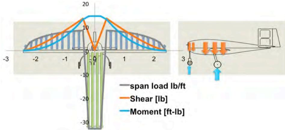
**Figure 5.1: Shear and moment diagram**
