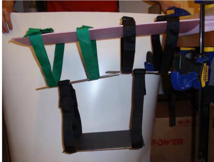
Figure 31: Half-Wingspan Wiffletree Test
