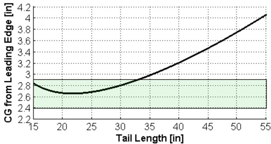
Figure 9: Center of Gravity Location for Each Tail Length
