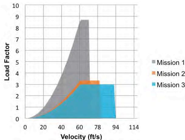
**Figure 5.2: V-n diagram**
