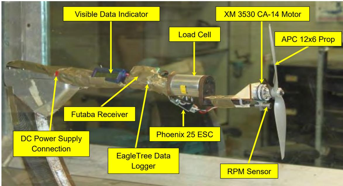
**Figure 54: Picture of Propulsion Wind Tunnel Test**
