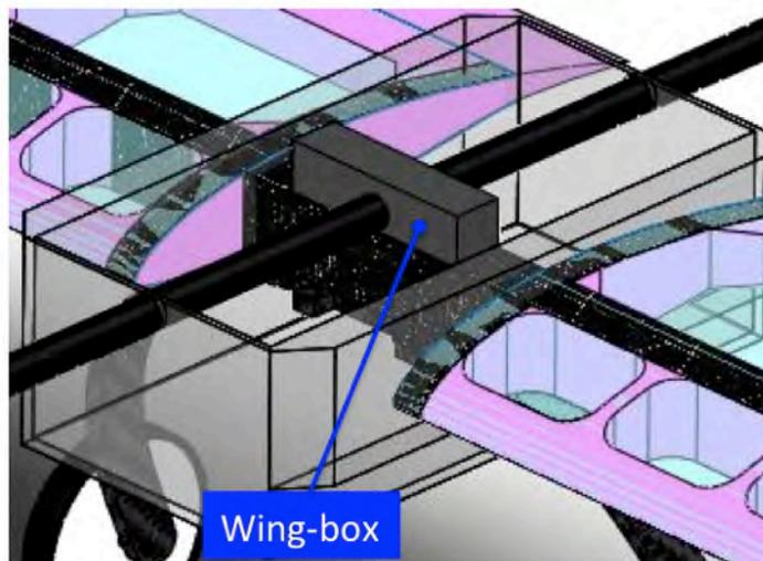
**Figure 5.5: Wing-box placement**
