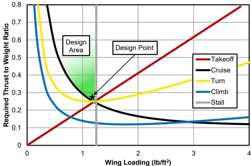
**Figure 12: Thrust to Weight vs. Wing Loading**
