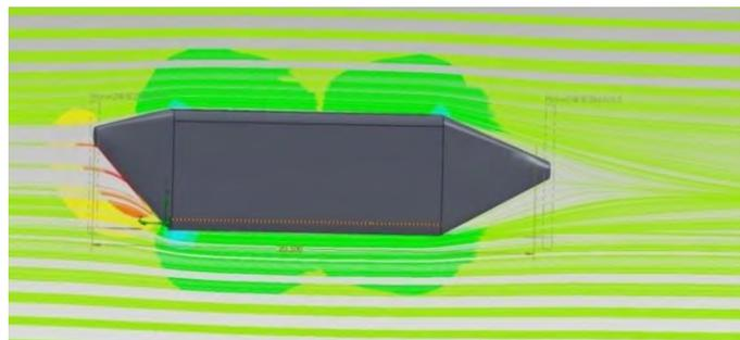
Figure 17: Fuselage Flow Simulation (10)
