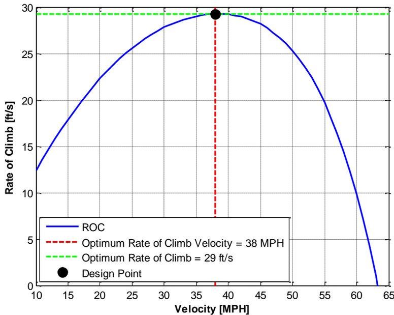
**Figure 29: Optimized Rate Of Climb as a Function of Velocity**
