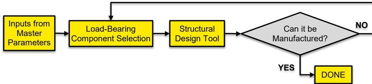
**Figure 26: Structural Design Process**
