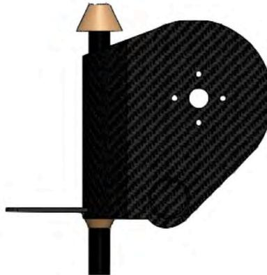
**Figure 5.11: Off set motor mount with nose gear attachment included**
