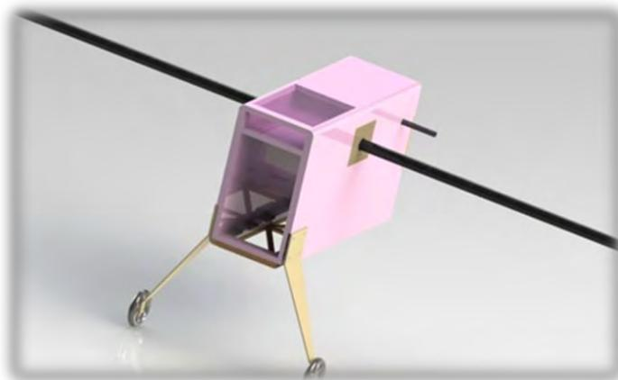
Figure 24: Foam Fuselage
