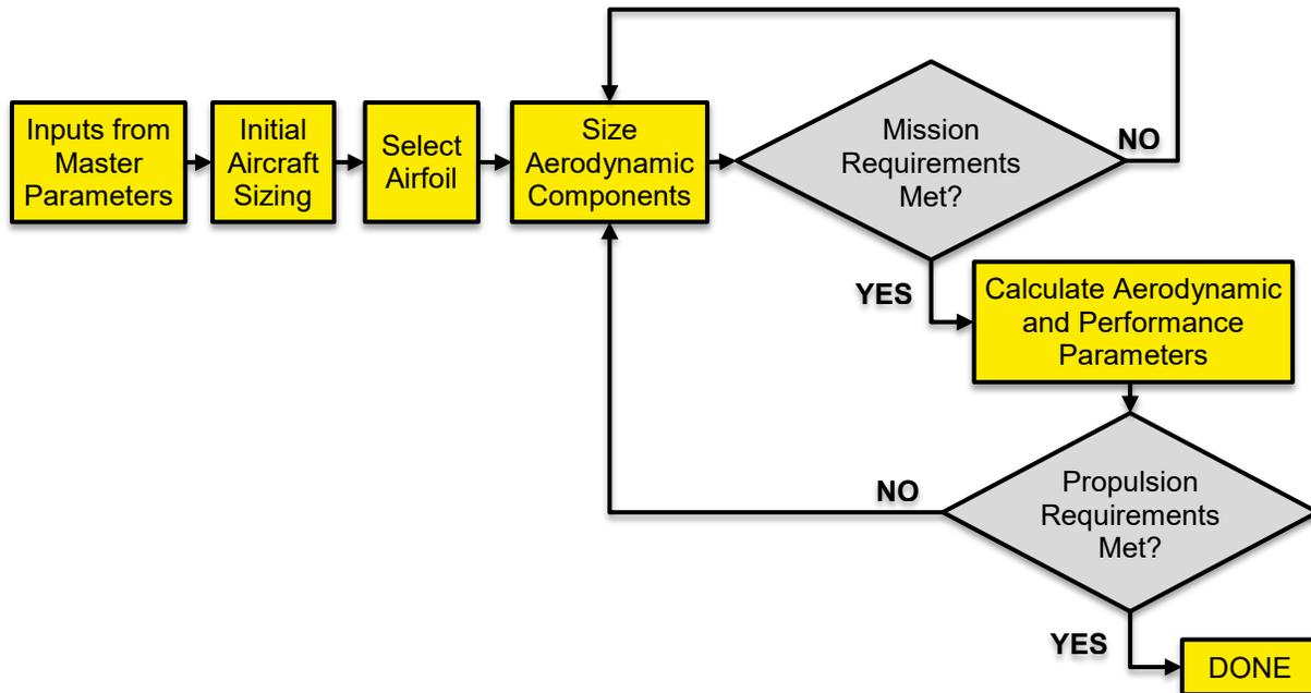
**Figure 13: Aerodynamics Design Process**
