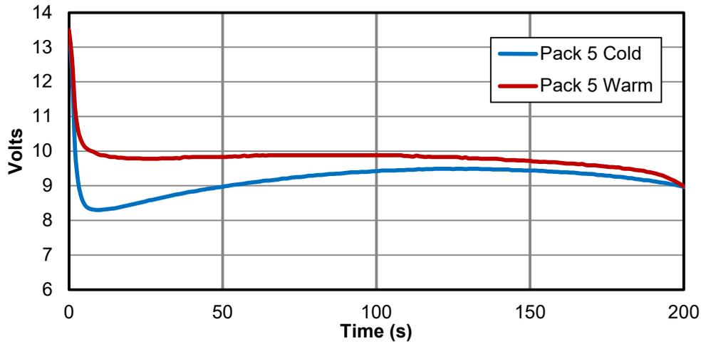
**Figure 52: Cold Battery 20A Discharge Test**
