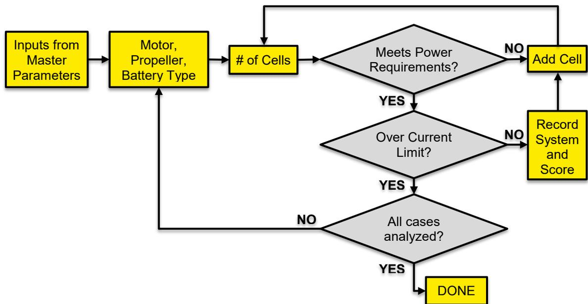
**Figure 21: Propulsion Design Process**
