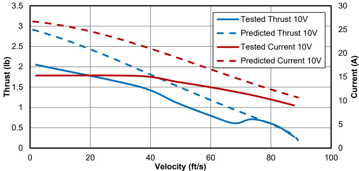
**Figure 65: Thrust profile comparison**
