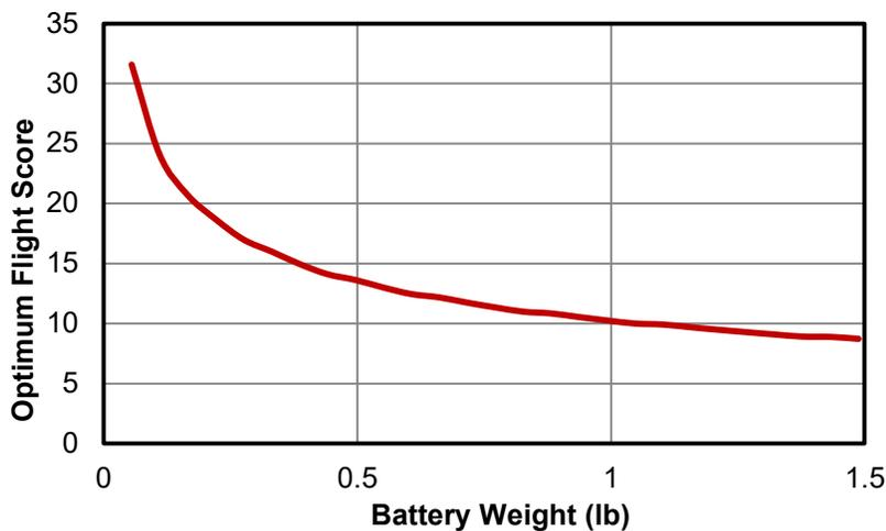
**Figure 4: Optimum Flight Score vs Battery Weight**
