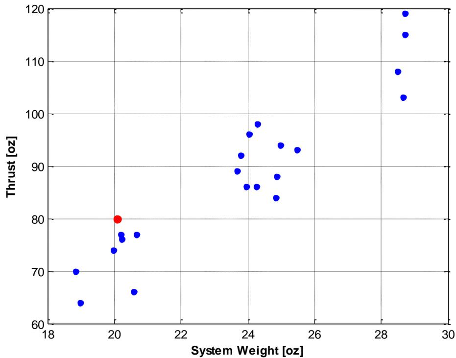
**Figure 11: Propulsion System Weight vs. Theoretical Electricalc (7) Thrust for 25 Different Commercially Available Brushless Motors**
