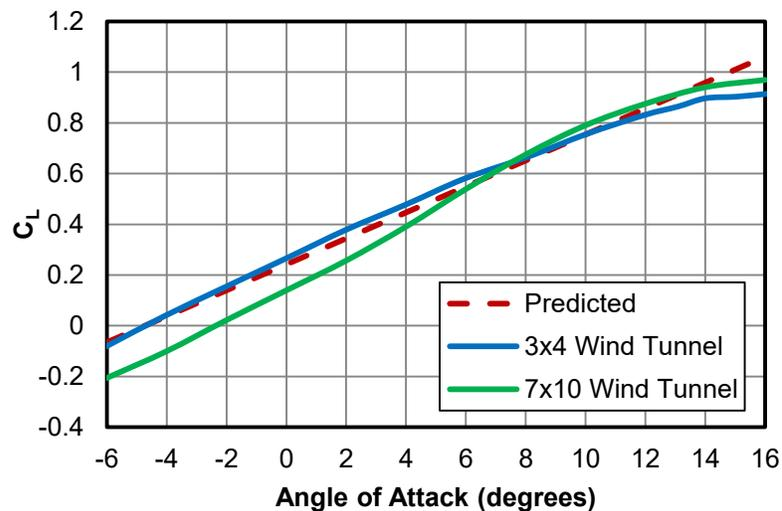
**Figure 61: Lift Curve Slope Comparison**
