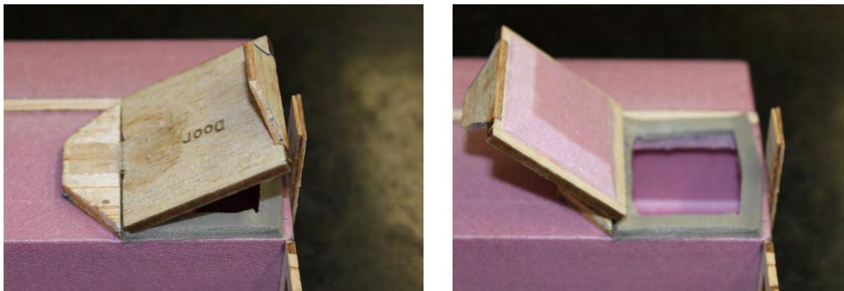
**Figure 38: Dump Valve Showing Foam-to-Weather Stripping Seal**
