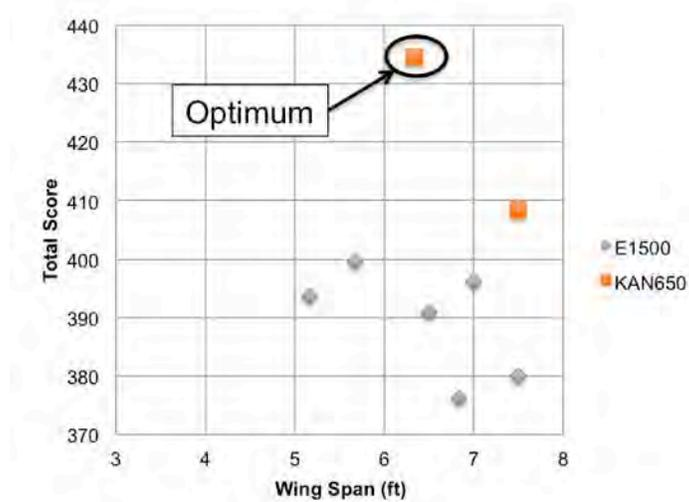
**Figure 4.6: Effects of battery selection and span on total score**
