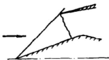
Figure 5.2 external compression inlet
