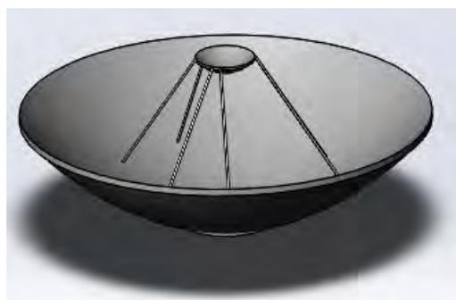
**Figure 5.4-1** *3.0-meter Parabolic HGA*
