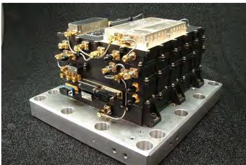
**Figure 5.4-2** *Electra UHF Radio*
