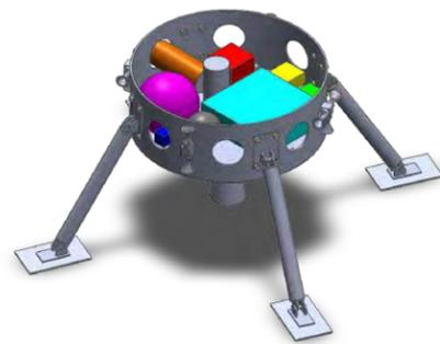
**Figure 3.5-1** *Isometric View of the Vespucci Stowed Configuration*
