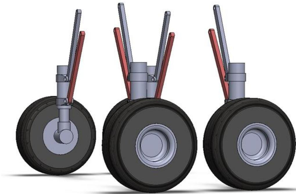
**Figure 12-2 Main Landing Gear**
