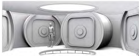
External transfer floor with CBM airlock hatches
