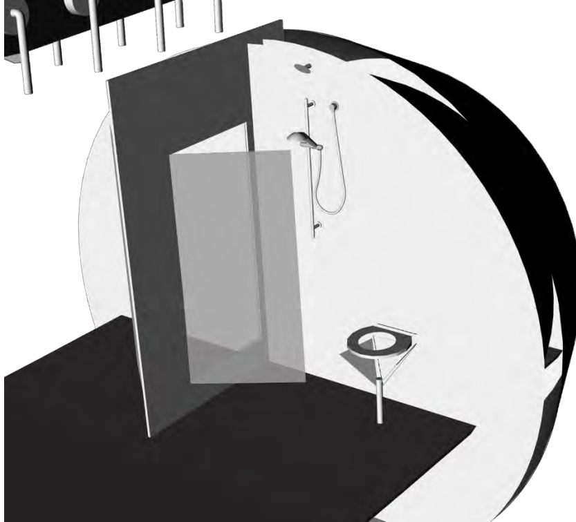
Figure 32: The restroom installed on both Module 1 and Module 2 feature a detachable showerhead so as to allow crewmembers complete control of the flow of water in response to the unnatural Coriolis effects
