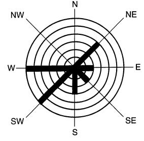
In the illustration, the wind blew from the west 6 times; from the southwest 6 times; from the south 3 times; and from the southeast and east 2 times; and from the northeast 4 times each (a total of 23 observations). The wind rose shows that in this case, west/southwest winds dominate. You could make several wind roses to determine how the wind pattern in your area changes throughout the year.
