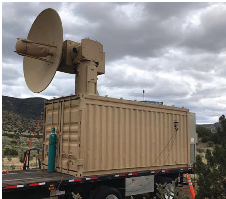
▲ The Tactical High-Power Operational Responder was developed to defend air bases against swarms of drones.
