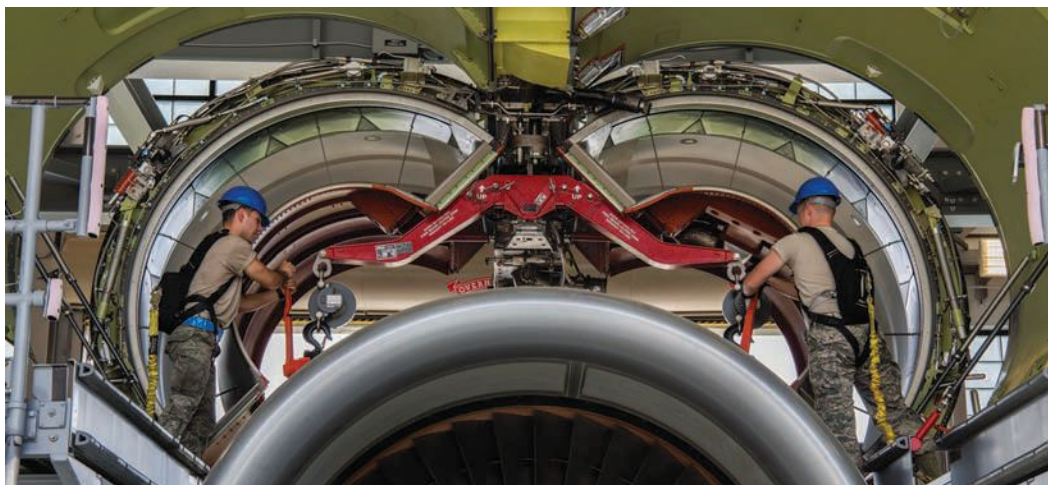
◀ Airmen lower an engine from a C-5M Super Galaxy cargo jet for maintenance at Dover Air Force Base, Del. More efficient tools developed by the non-deterministic approaches community are maximizing the service life and safety of jet engines.
