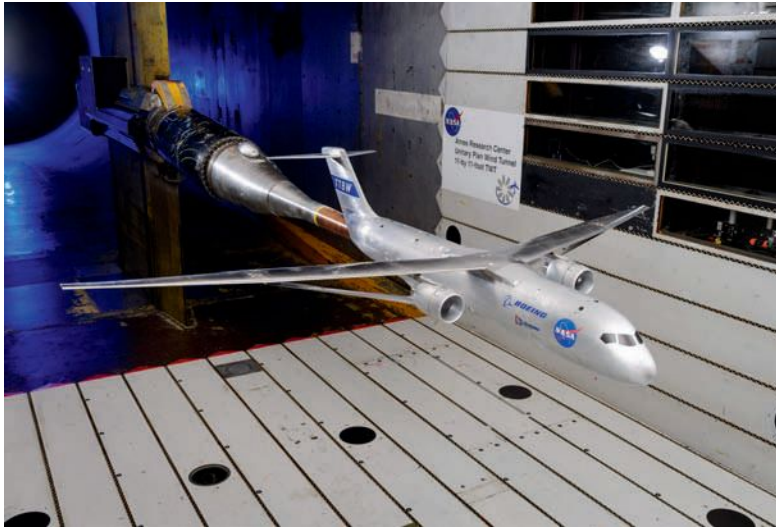
▲ A NASA-Boeing 4.5% scale of a Transonic Truss-Braced Wing aircraft is tested in the 11-Foot Transonic Tunnel at NASA's Ames Research Center. Boeing/NASA
