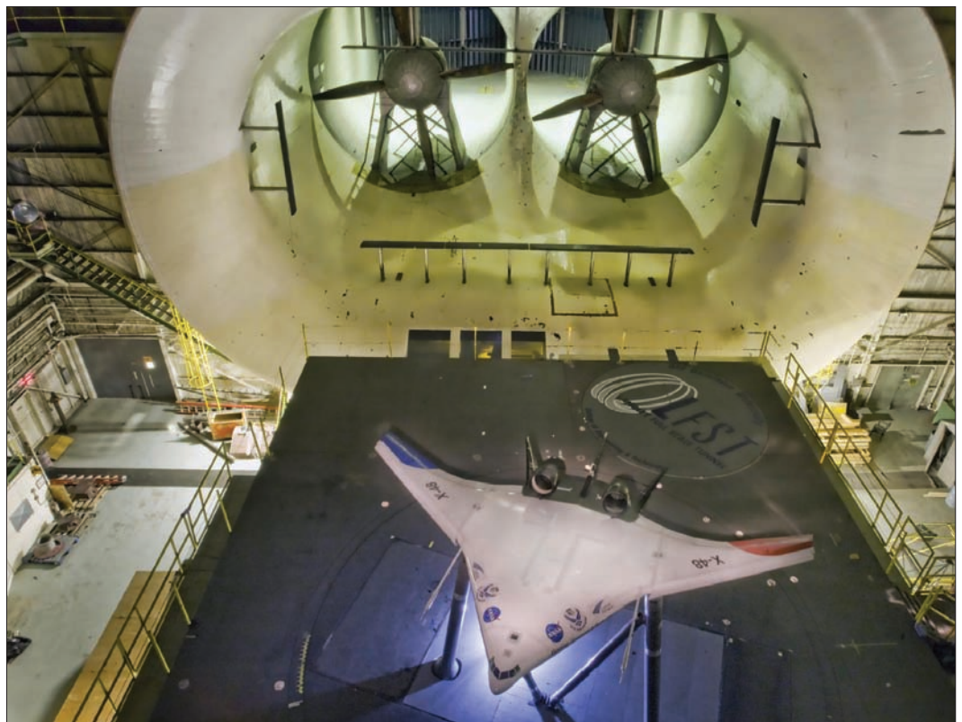
An X-48C is mounted in the recently dismantled Full-Scale 30x60-ft Wind Tunnel. USAF photo by Staff Sgt. Barry Loo.
