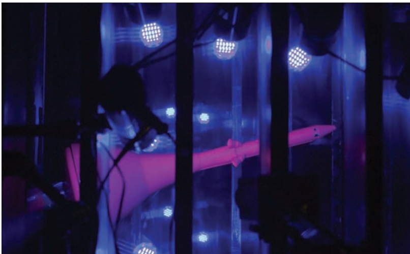
A 5% scale model of the Orion launch abort vehicle was installed in Langley’s Unitary Plan Wind Tunnel for supersonic jet effects testing. The model was painted with pressure-sensitive paint and illuminated to produce surface static pressure maps in the locations of the attitude control motor nozzles and the aft-body interaction regions.
