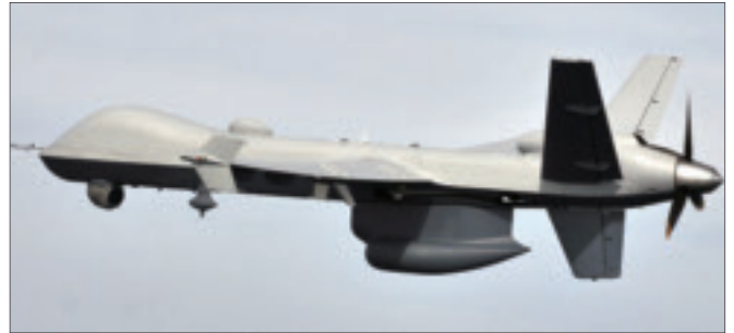
The SeaVue SAR/ISAR and an over-water-optimized MTS-B EO/IR sensor were mounted in the belly of a Guardian UAV for the CBP.
